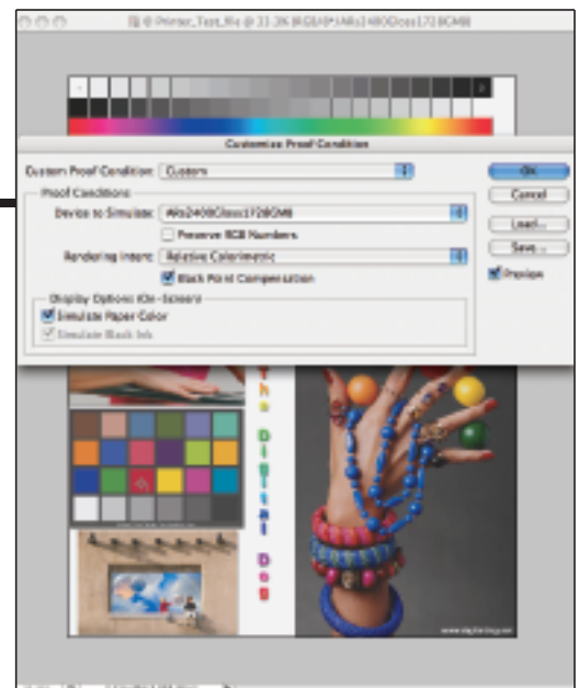
Figure 2. Here is a soft proof setup for my Epson Stylus Photo R2400 with the Simulate Paper Color and Ink Black display options on. These settings render the soft proof in the background a bit flat looking.
