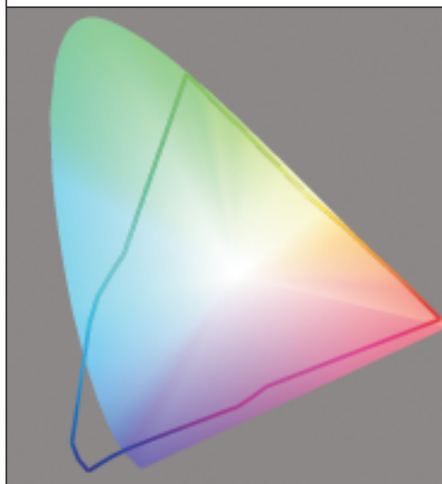
Figure 1. In this 2D gamut plot in ColorThink, you can see the huge gamut of ProPhoto RGB—so big that the blue primary falls outside the range of human vision, as represented by the horseshoe plot.
