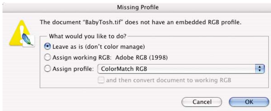
Fig. 9-6-2 The Missing Profile dialog appears because BabyTosh.tif has no embedded profile. The profile seen in the Assign Profile pop-up menu may not match the profile you see since the last selected profile appears here.
