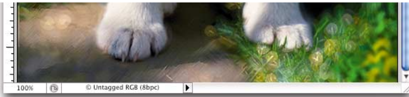
Fig. 9-6-3 After BabyTosh.tif is open, the Profile indicator shows that this is an untagged document.
