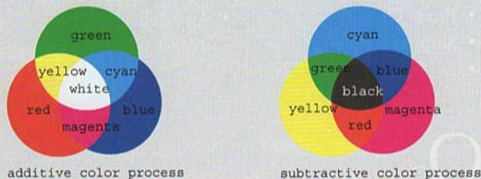
Figure 1. Both the additive and subtractive color models are seen here. RGB or additive colors are based on the mixing of light. CMYK colors are based on removing light from a page by adding colorants.
