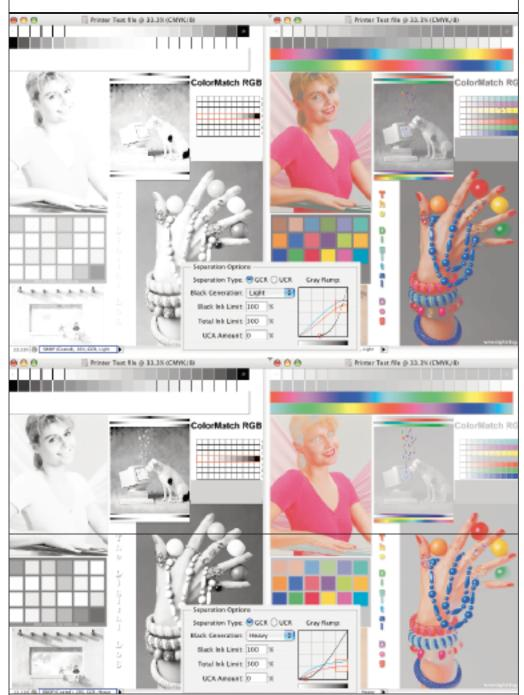
The effect of GCR on the black channel and CMY channels in Photoshop. Notice how a light GCR produces a fainter black channel, indicating that more CMY inks are used to produce the same colors. The opposite is the case with high GCR. You can use Photoshop's Custom CMYK engine to test this yourself once you set the Separation Options as pictured.
