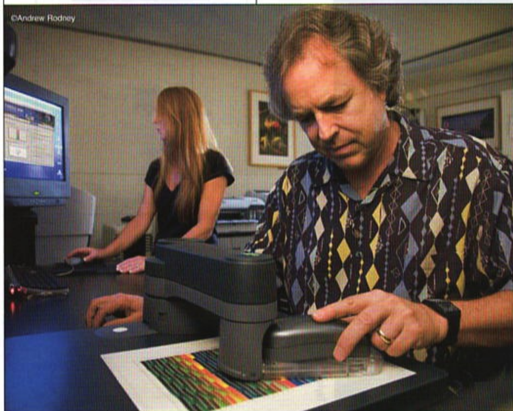
Mac Holbert sets up the Eye-One iO to measure a target for building a custom ICC paper profile.
